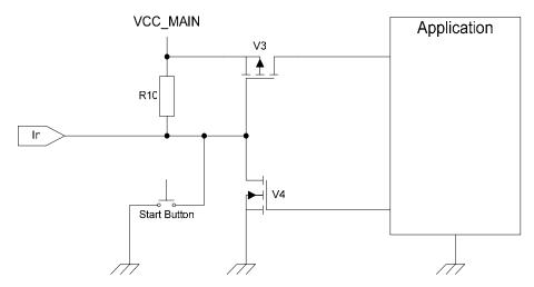
Figure 5.20-3 Example of host wake-up circuit
